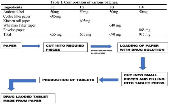
Figure 1. Steps involve in production of paper tablet.
