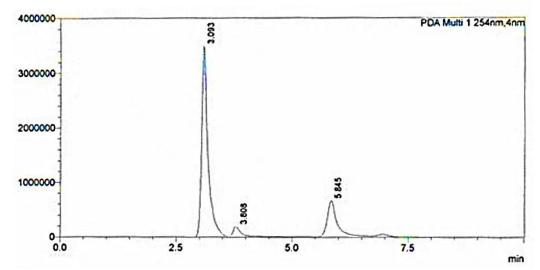
Figure 1. Chromatogram optimization of mobile phase comparison (methanol: water) 70:30, flow rate 1 mL/minute and column temperature 30°C.
