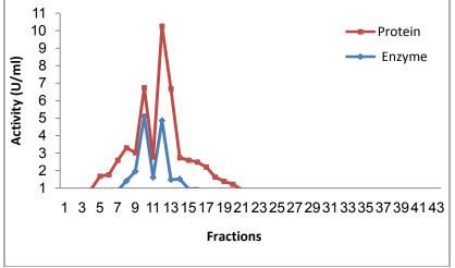
Figure 1. Elution Profile of Sephadex G-100 fraction ion exchange Column Chromatography. An Aliquote of Each Fraction was assayed for Protein Content and Tyrosinase Activity. Tyrosinase Eluted with Linear Gradient of Potassium Phosphate Buffer at 0-100 mM.
