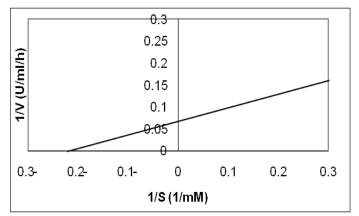
Figure 4. Lineweaver-Burk plot relating the reaction velocity of *S. cerevisiae* tyrosinase to substrate concentration.
