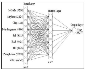
Figure 1. Layers and connection of a feed-forward backpropagating ANN. The neural network model developed here applies the sigmoid transfer function to compute the strength of interconnection between each pair of neurons.
