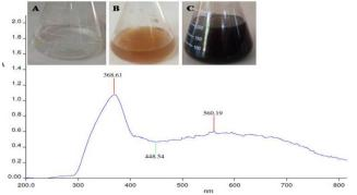
Figure 1. Visual observation (A) Silver solution (B) plant extract (C) synthesis of silver nanoparticles and UV -vis spectra shows effect of synthesis of *Melia azedarach* leaf extract mediated silver nanoparticle.
