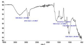
Figure 2. FTIR spectrum of silver nanoparticles synthesized by leaf extract of (A) *Melia azedarach* (B) Silver nanoparticles.
