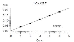
Figure 1. The calibration curve of calcium standard solution.
