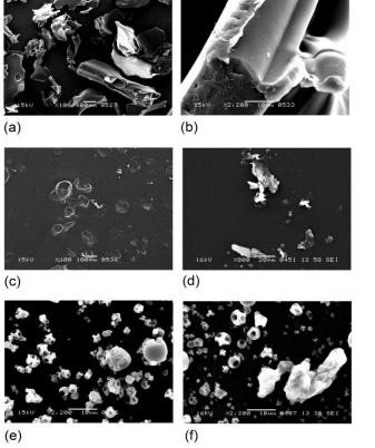
Figure 4. SEM images of (a,b) 'as received' PVP, (c,d) 'as received' *o*-carborane, (e) spray-dried PVP (sample #4, inlet temperature 180 °C), (f) co-spray-dried PVP/*o*-carborane (sample #13, inlet temperature 180 °C); magnification (a)  $100\times$ , (b)  $2200\times$ , (c)  $100\times$ , (d)  $800\times$ , (e)  $2200\times$ , (f)  $2200\times$ .
