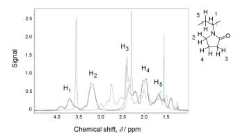
Figure 1. <sup>1</sup>H NMR spectra of 'as received' *o*-carborane (blue), 'as received' PVP (green), spray-dried PVP (2 %w/v; brown) and co-spray-dried PVP (2 %w/v) with *o*-carborane (0.2 %w/v; purple). Labels refer to hydrogen atoms in the PVP structure shown, with peak assignments having been made in [37].
