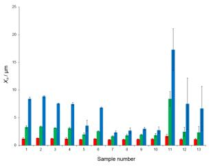
Figure 3. Mean particle diameters of spray-dried PVP and co-spray-dried PVP/o-carborane samples: red =  $x_{10}$ , green =  $x_{50}$ , blue =  $x_{90}$  values; particles determined using spray drying (mean  $\pm$  SD, n = 3).
