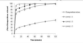
Figure 3. Release profiles of DMP from the different drug adsorbates with Aerosil 200 in comparison with the pure drug.
