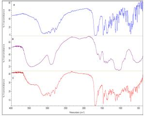
Figure 1. FT-IR spectra of DMP (A), HPMC 15000 (B) and 1:1 (w/w) physical mixture of them (C).
