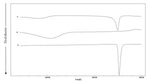
Figure 2. DSC thermograms of DMP (A), HPMC 15000 (B) and 1:1 (w/w) physical mixture of them (C).
