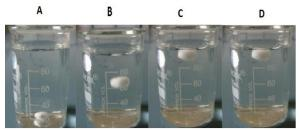
Figure 4. Floating process for a tablet containing 40% Na Alg during lag time (A), the start of floating process (B), during floating time (C) and after 12 hours testing (D).
