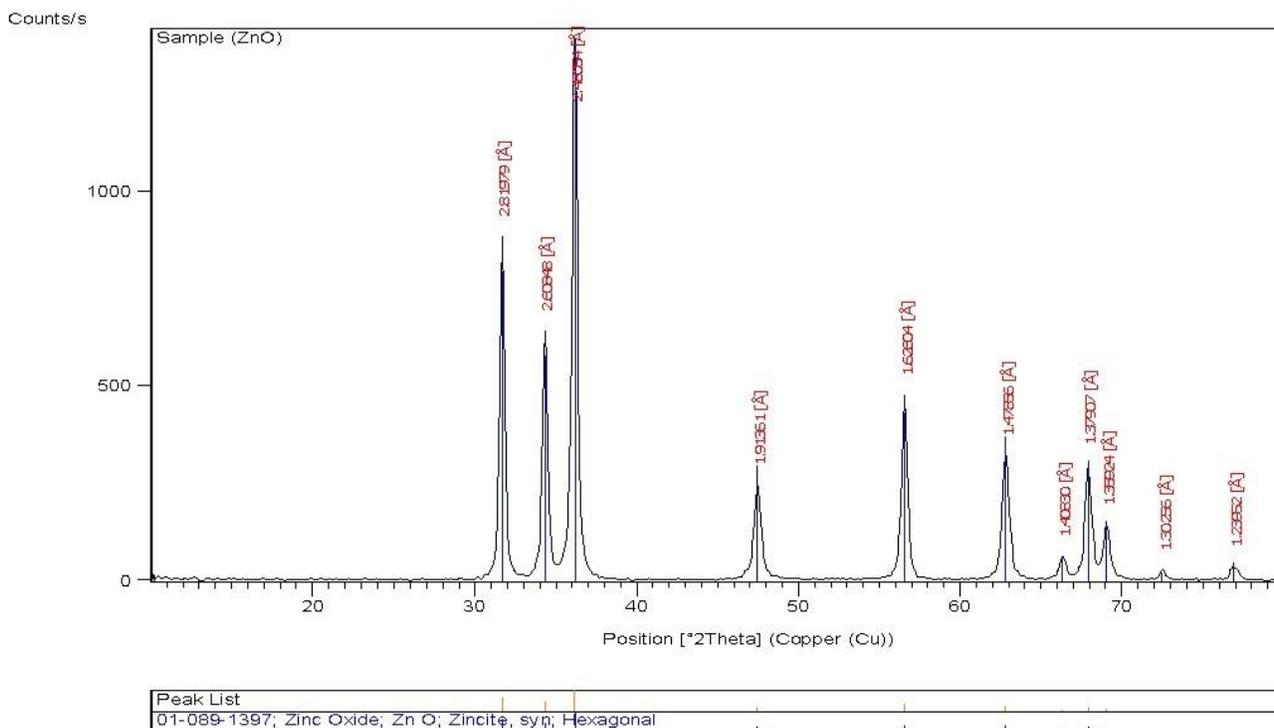
Figure 3. The X-ray diffraction graph refers the purity and crystallite size of ZnO NPs @ PEG.
