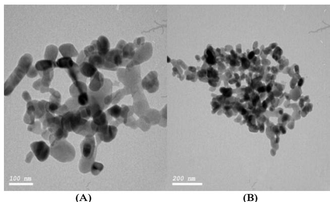
Figure 1. (A) and (B) different spots of transmission electron microscope (TEM) imaging taken with different magnification scales (100 and 200 nm) for ZnO NPs @ PEG.
