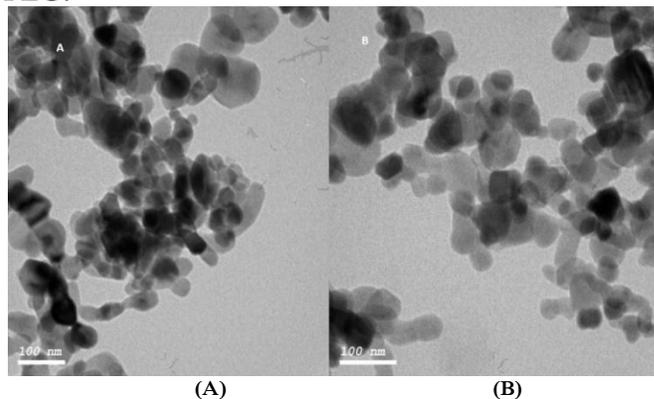
Figure 2. (A) and (B) different spots of transmission electron microscope (TEM) imaging taken with different magnification scales (100 and 200 nm) for ZnO NPs @ PVP.
