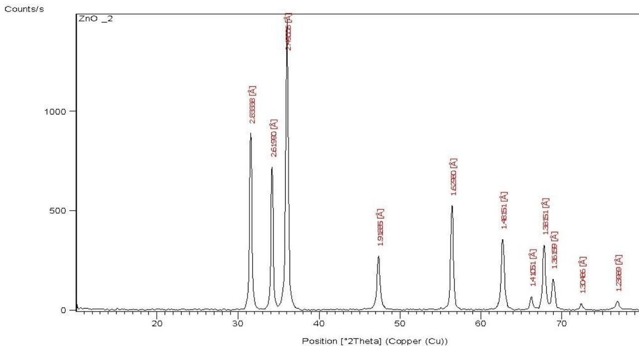
Figure 4. The X-ray diffraction graph refers the purity and crystallite size of ZnO NPs @ PVP.
