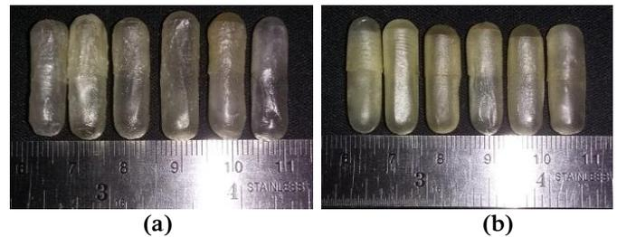
Figure 1. Alginate-chitosan capsule shells crosslinked tripolyphosphate (a) formula F7; (b) formula F8
