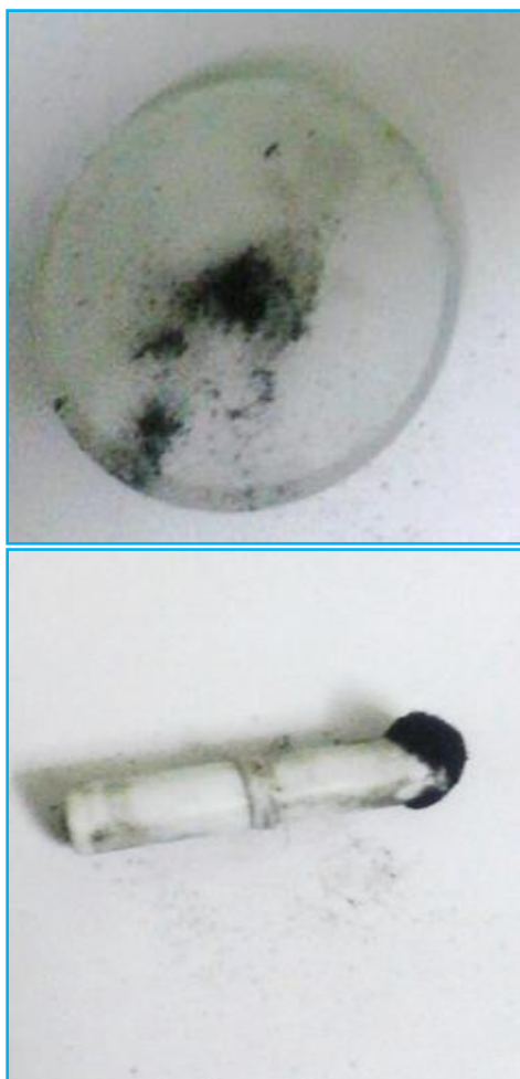
Figure 2. Purified magnetic iron oxide nanoparticles and its aggregation towards the magnetic bead.
